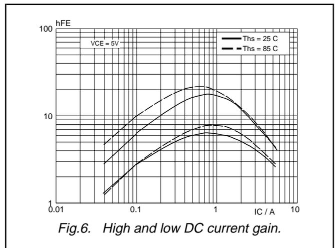
Fig.6. High and low DC current gain.
