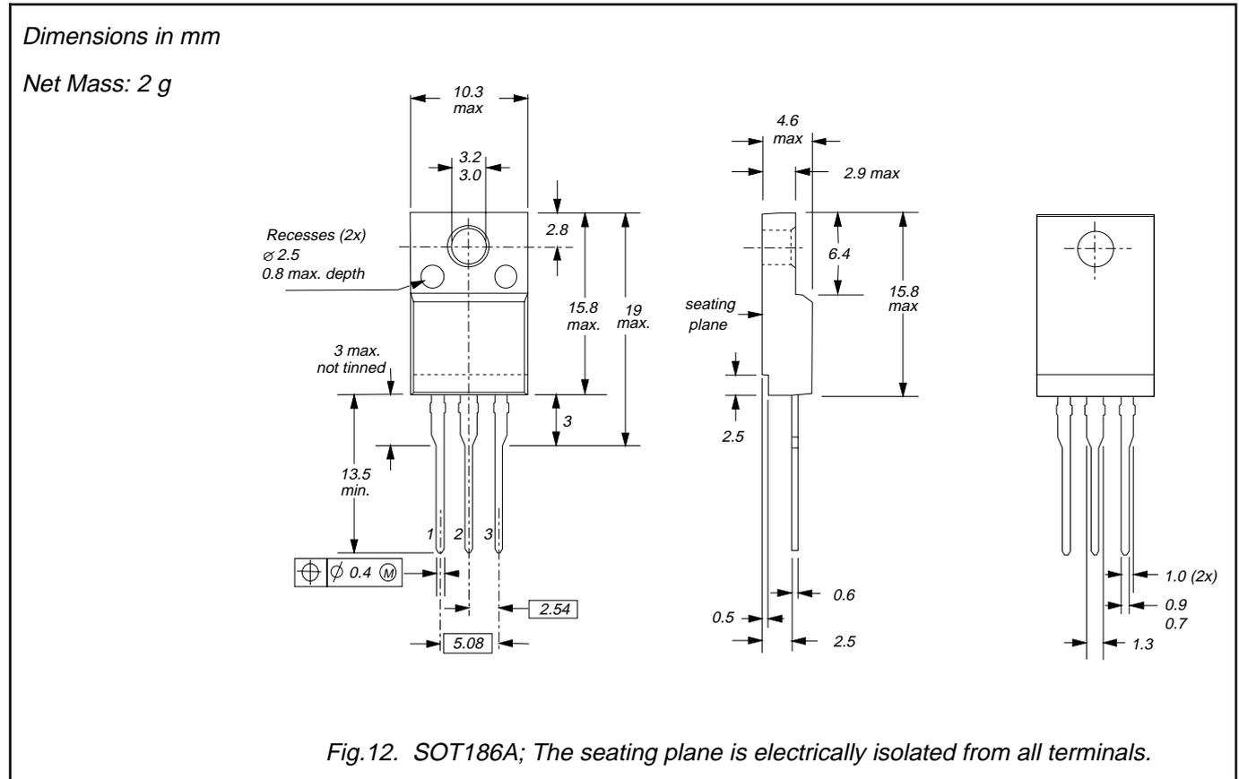
Fig.12. SOT186A; The seating plane is electrically isolated from all terminals.
