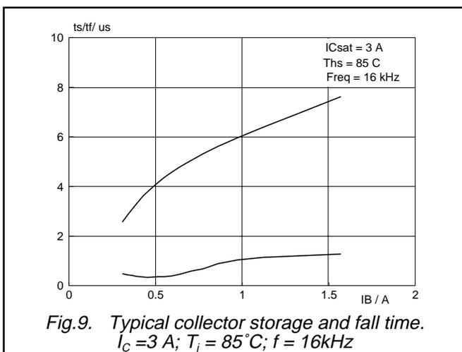
Silicon Diffused Power Transistor
