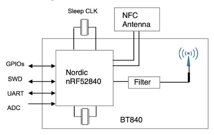
BlurNor BT840F is a sister module of BT832F. The physical size is the same. There are 21 additional LGA pins for additional GPIOs provided by nRF52840.
