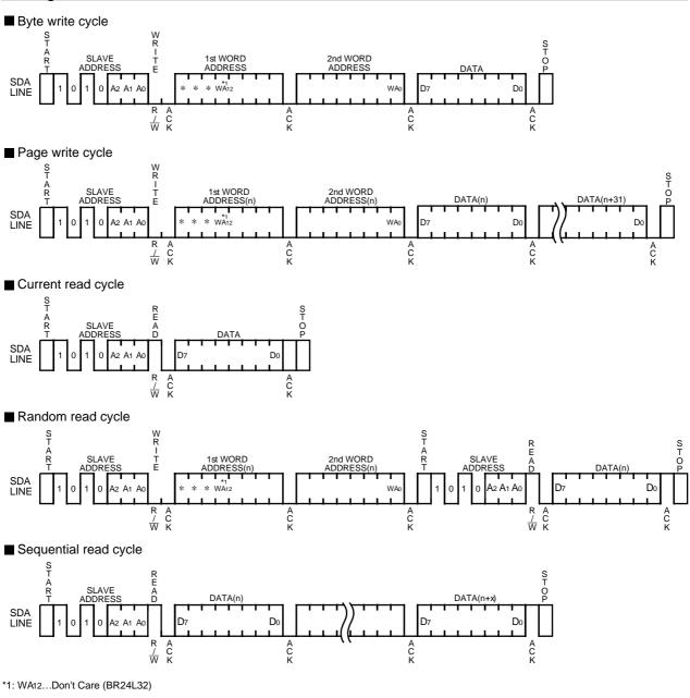
Note : BR24C32/F has no letter "-W", but it is a double-cell type. BR24C64/F is a single-cell type. Please be careful not to confuse w-cell type and single-cell type. ("-W" means double-cell type.)
