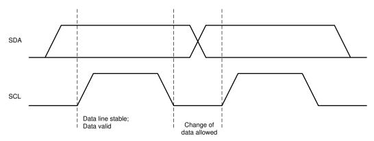
Figure 29. Bit Transfers on the I<sup>2</sup>C Bus
