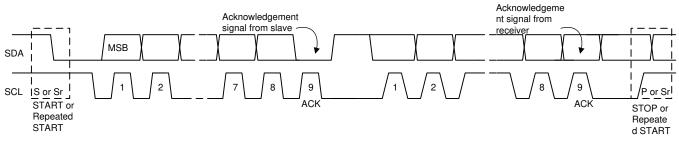
Figure 31. Data Transfer on the I<sup>2</sup>C Bus
