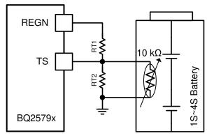
Figure 25. TS Resistor Network
