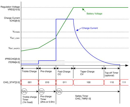
Figure 23. Battery Charging Profile
