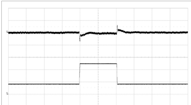
Output voltage response to load current step change (25%–75%–25%) at V_i = 12 V, C_{OUT} = 8 \times 330 \mu F / 10 \text{ m}\Omega + 20 \times 100 \mu F , di/dt = 2 \text{ A}/\mu s , ACSR Gian=219 and ASCR Residual=82. Scale from top: 50 mV/div, 20 A/div, 500 \mu s /div. Note: Sense pins are connected to load.
