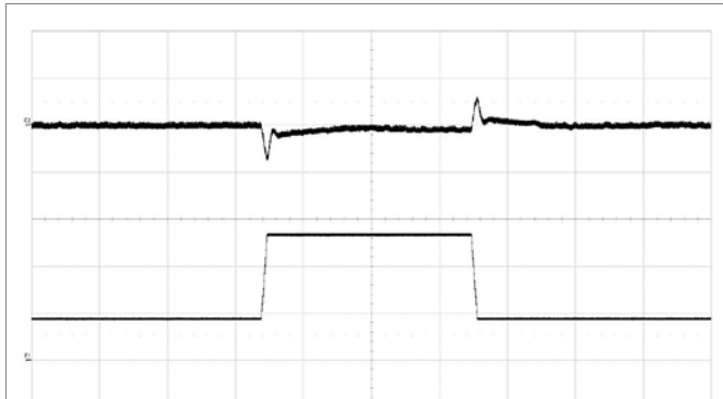
Output voltage response to load current step change (25%–75%–25%) at V_i = 12 V, C_{OUT} = 8 \times 330 \mu F / 10 \text{ m}\Omega + 20 \times 100 \mu F , di/dt = 2 \text{ A}/\mu s , ACSR Gian=219 and ASCR Residual=82. Scale from top: 50 mV/div, 20 A/div, 200 \mu s /div. Note: Sense pins are connected to load.
