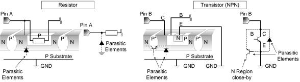
Figure 19. Example of monolithic IC structure
