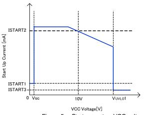
Figure 5. Start current vs VCC voltage
