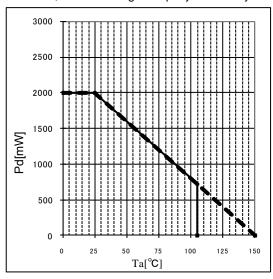
Figure 18. Thermal Abatement Characteristics
