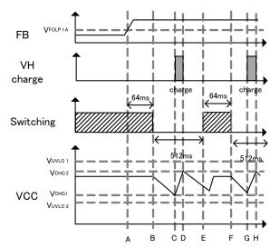
Figure 15. Over load protection (Auto recovery)
