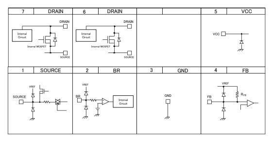
Figure 2. I/O Equivalent Circuit Diagram
