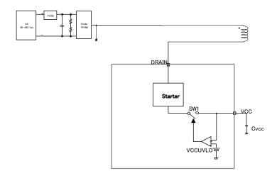
Figure 4. Block diagram of start circuit
