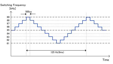
Figure 10. Frequency hopping function
