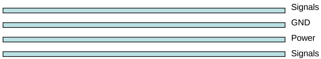
Figure 15: Typical 4-layer PCB construction
