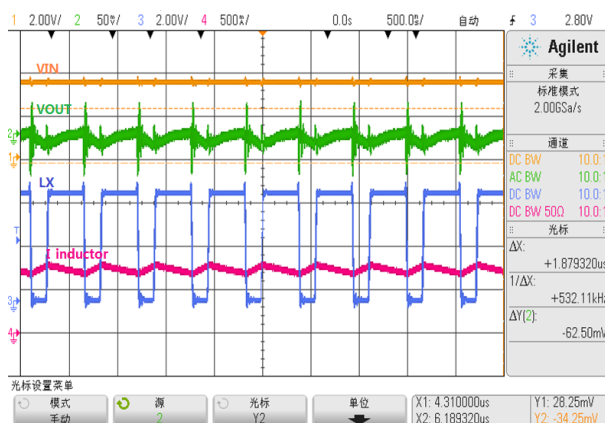
Output Ripple / LX / Inductor Current Vin=3.6V, Vout=5V, Iout=0.5A
