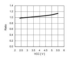
Fig.9 IOUT VCC dependency
