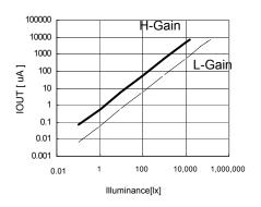
Fig.3 Illuminance - IOUT Characteristics
