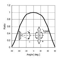
Fig.5 Directional Characteristics 2
