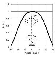
Fig.4 Directional Characteristics 1
