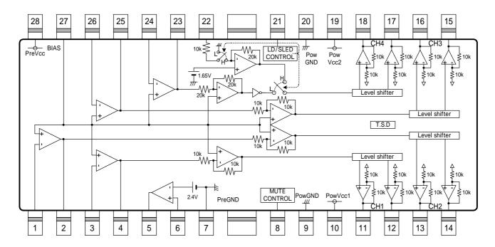
$$\label{eq:total_control} \begin{split} & \text{T.S.D}: \text{Thermal shutdown} \\ & \text{Resistance unit} : \left[\Omega\right] \end{split}$$
