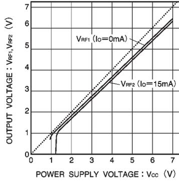
Fig.4 Output voltage vs. power supply voltage
