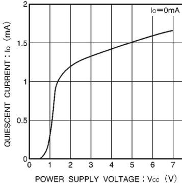
Fig.3 Circuit current vs. power supply voltage
