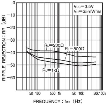
Fig.6 Ripple rejection vs. frequency
