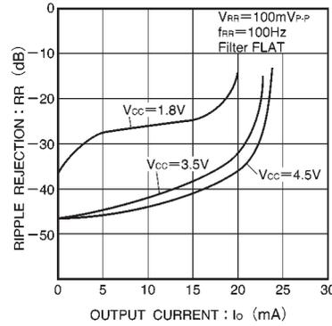
Fig.7 Ripple rejection vs. output current
