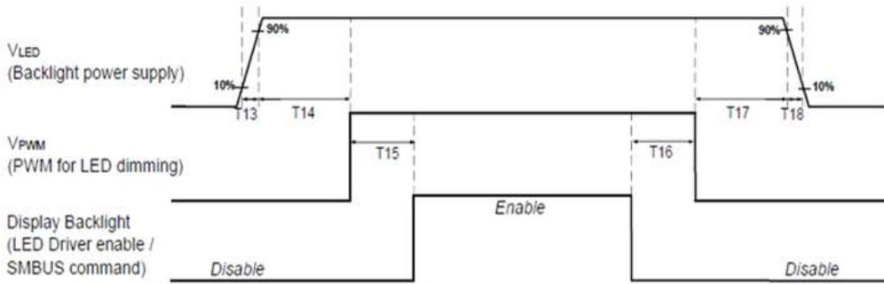
Note : When the adapter is hot plugged, the backlight power supply sequence is shown as below.
