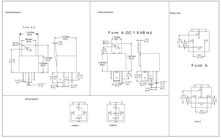
Dimensions in inches with millimeters in brackets below. Tolerance: ± .010"
