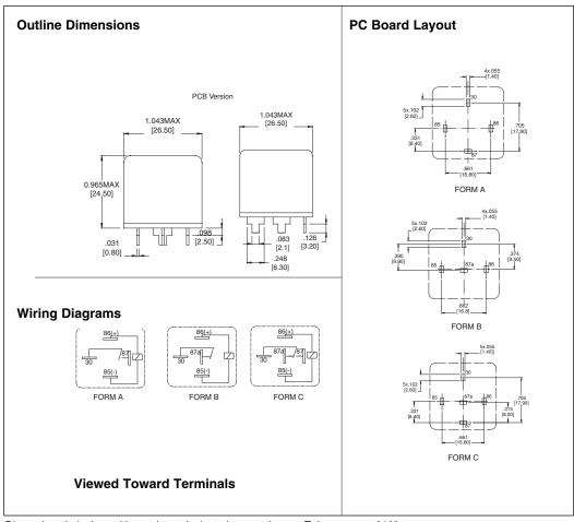
Dimensions in inches with metric equivalents in parentheses. Tolerance:  $\pm$  .010"
