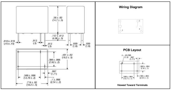
Dimensions in inches with metric equivalents in parentheses. Tolerance:  $\pm$  .010"
