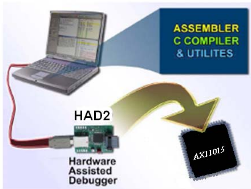
Figure 14: Typical Debugger and Hardware Assisted Debugger (HAD2) System Diagram
