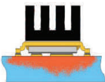
⑨ Mounted to a PCB with small clip heatsink (still air)
