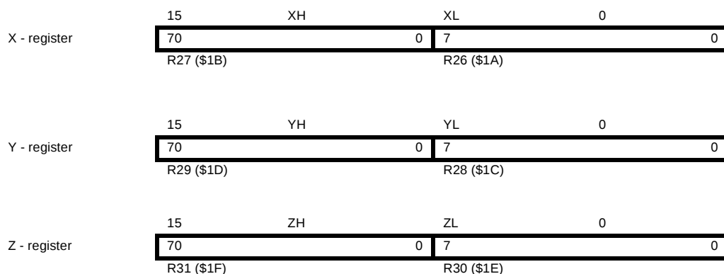
Figure 8. The X-, Y-, and Z-registers
