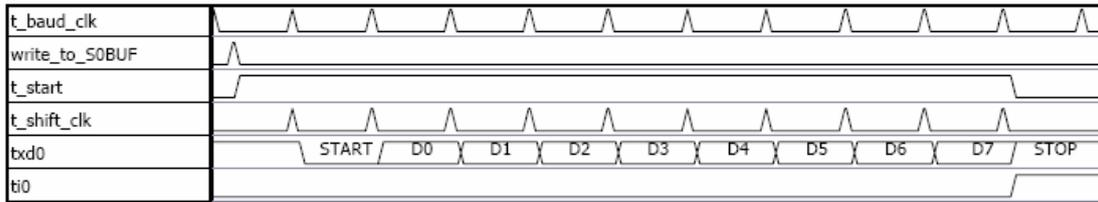
Figure 67. Serial0 transmission in mode 1
