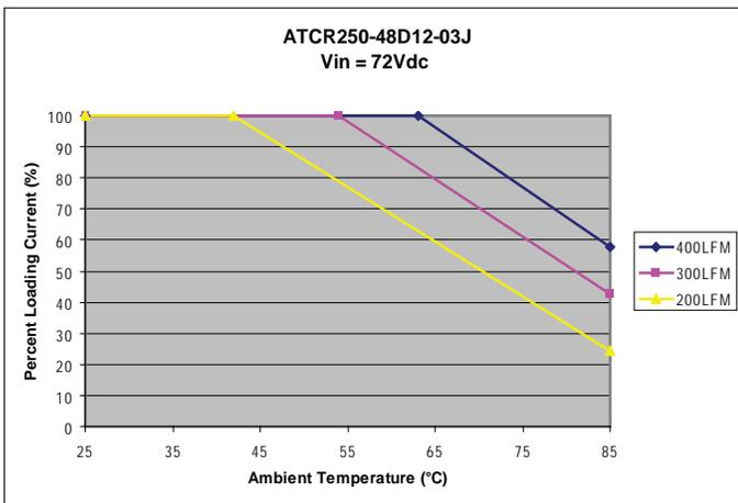
Figure 3: Derating Curve with Forced Air
