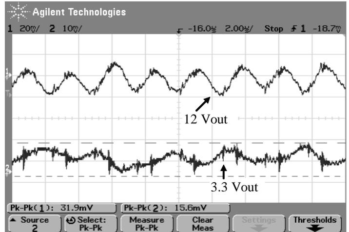
Figure 8: Typical Output Ripple and Noise Measurement
