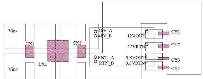
Figure 19: Conducted EMI filter recommended layout
