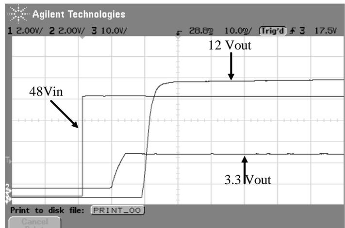
Figure 6: Turn-On Characteristic (48 vin)
