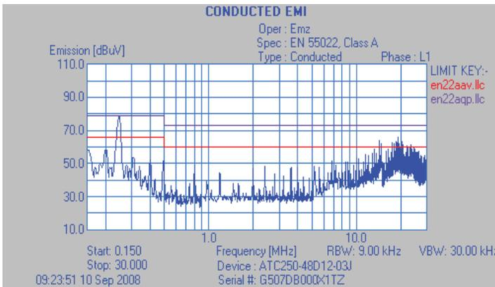
Figure 18: Class B Test Filter with Capacitors & Common\_mode choke
