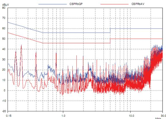
Figure 20: Typical Spectrum of the ATCR250 Test circuit as per Figure 18 & 19
