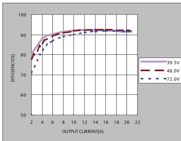
Figure 5: Efficiency vs. Load
