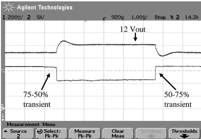
Figure 13: Typical Transient Response 75-50% and 50-75%
