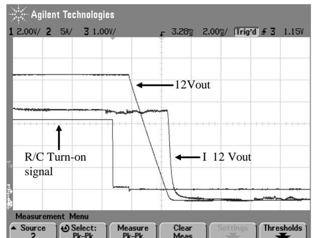
Figure 12: Remote Control Turning-off Characteristic
