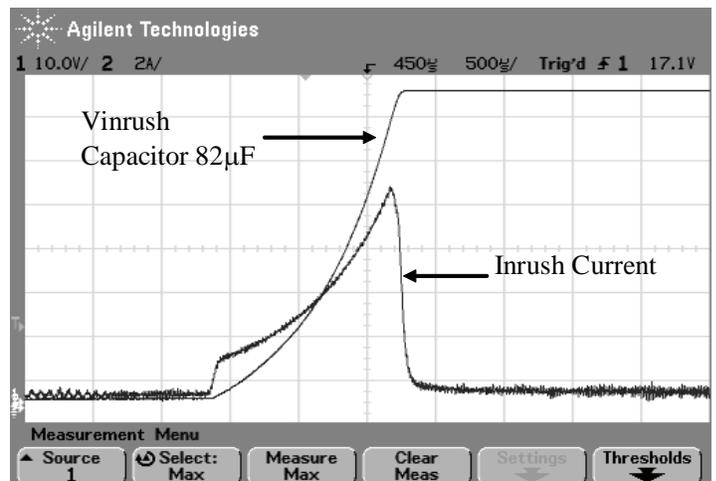
Figure 10: Inrush Current (72 V)
