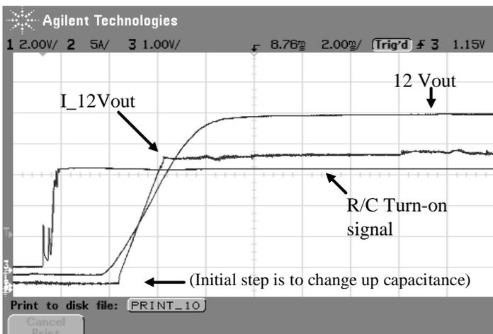
Figure 11: Remote Control Turning-on Characteristic
