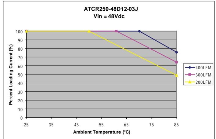
Figure 2: Derating Curve with Forced Air
