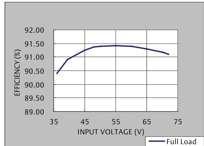
Figure 4: Efficiency vs. Line (Full Load)
