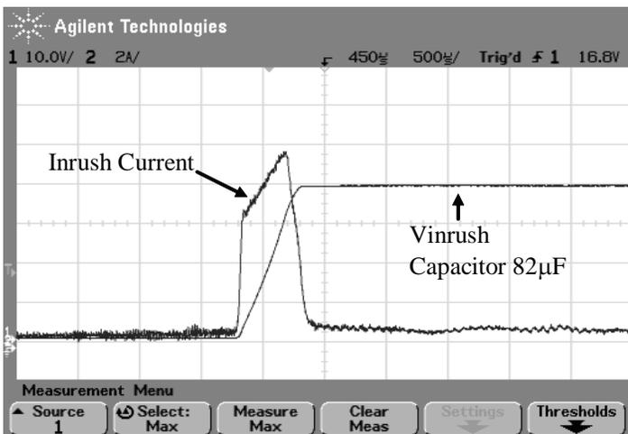
Figure 9: Inrush Current (39.5 V)
