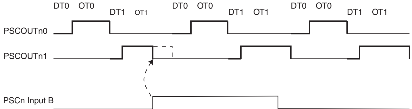
Figure 12-36. PSC behavior versus PSCn Input B in Mode 9.
