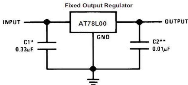
\*Required if the regulator is located more than 3" from the power supply filter.
