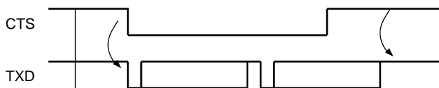
Figure 21-28. Transmitter Behavior when Operating with Hardware Handshaking
