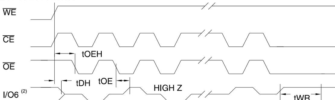
Notes: 1. Toggling either  $\overline{\text{OE}}$  or  $\overline{\text{CE}}$  or both  $\overline{\text{OE}}$  and  $\overline{\text{CE}}$  will operate toggle bit.
