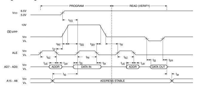
Notes: 1. The Input Timing Reference is 0.8V for  $V_{\rm IL}$  and 2.0V for  $V_{\rm IH}$ .
