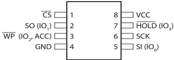
**Figure 1-2. 8-UDFN (Top View)**
