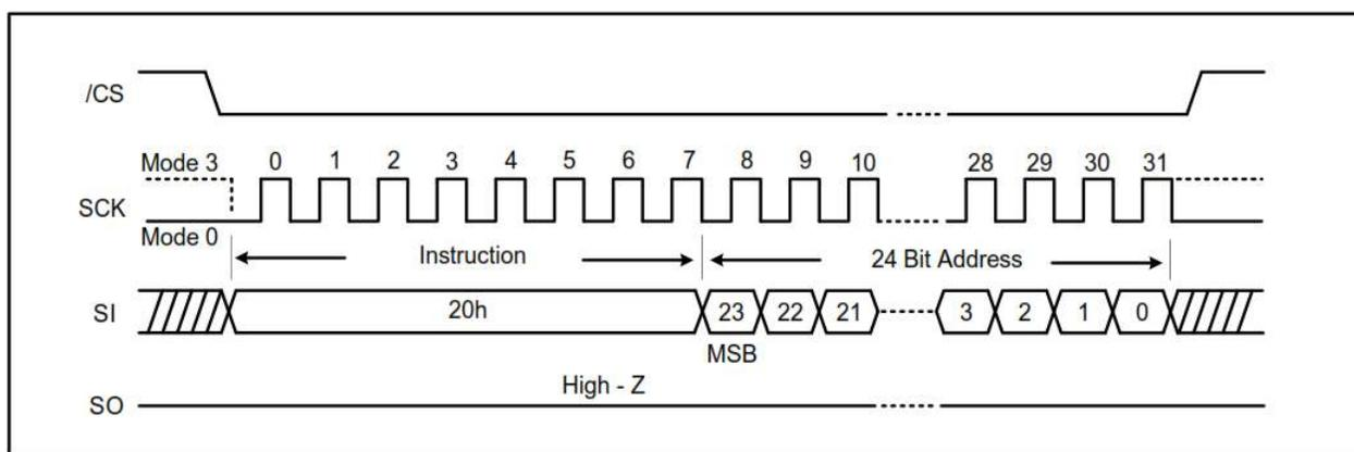
Figure 7-27. Block Erase Instruction (QPI Mode)
