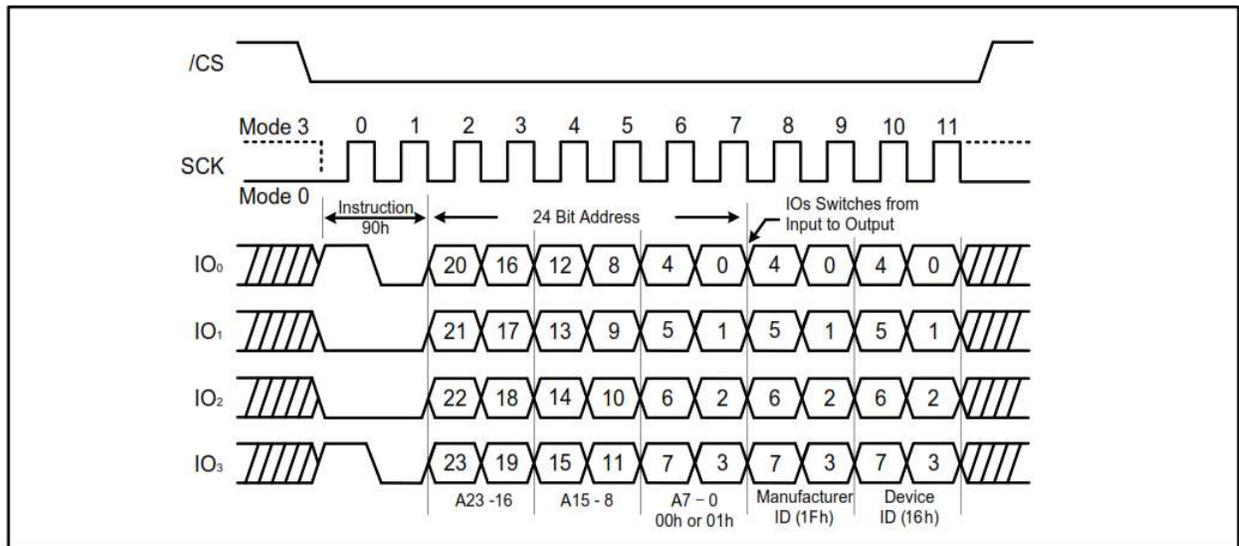
Figure 7-45. Read Quad Manufacturer/ Device ID Quad I/O instruction (SPI Mode)
