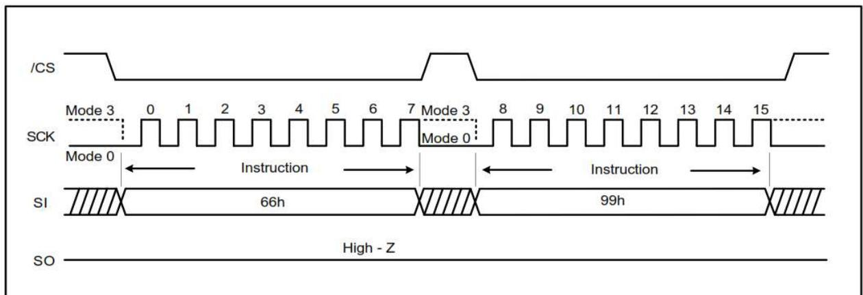
Figure 7-57. Enable Reset and Reset Instruction (QPI Mode)
