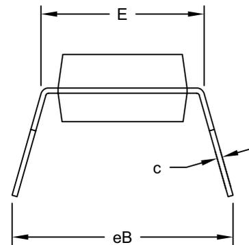
**8-Lead Plastic Dual In-Line (P) - 300 mil Body [PDIP]**
