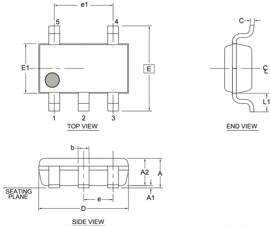
1. Dimension D does not include mold flash, protrusions or gate burrs. Mold flash, protrusions or gate burrs shall not exceed 0.15 mm per end. Dimension E1 does not include interlead flash or protrusion. Interlead flash or protrusion shall not exceed 0.15 mm per side.
