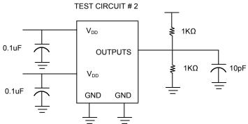
For parameter  $t_8$  (output skew rate) on -1H devices
