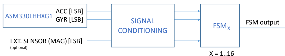
Figure 2. State machine in the ASM330LHHXG1
