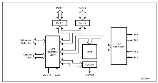
Figure 1. 82527 Block Diagram
