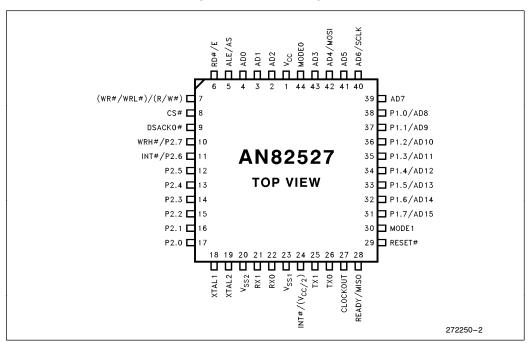
Figure 2. 44-Pin PLCC Package
