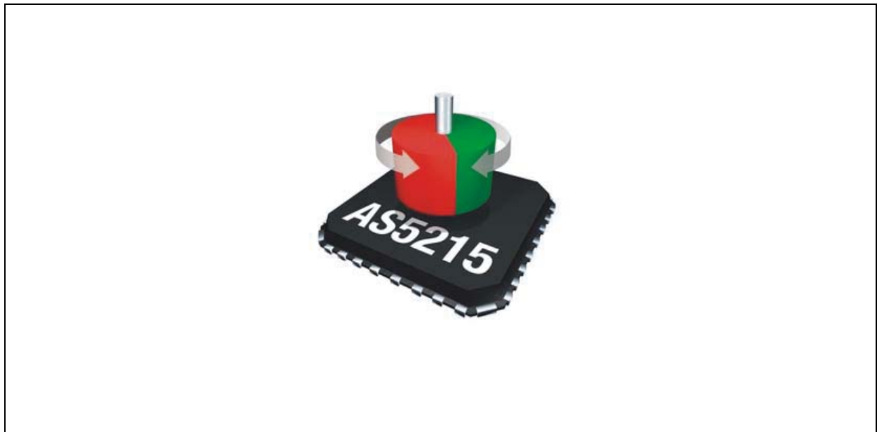
Figure 3. Typical Arrangement of AS5215 and Magnet
