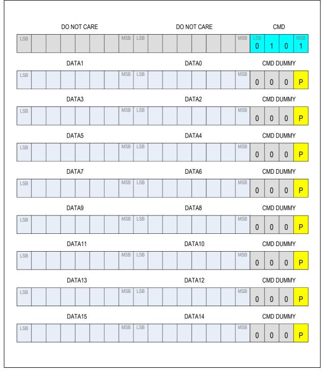
The command is composed by a first frame transmitted to the AS5165. The device is in slave communication mode. The device remains for the time TSW<sub>ITCH</sub> in IDLE mode before changing into the master communication mode. The AS5165 starts to send 8 frames. This command will read the SFRs. The numbering of the data bytes correlates with the address of the related SFR.
