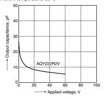
12.-(2) Output capacitance vs. applied voltage characteristics
