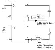
2) Even if spike voltages generated at the load are limited with a clamp diode if the circuit wires are long, spike voltages will occur by inductance. Keep wires as short as possible to minimize inductance.
