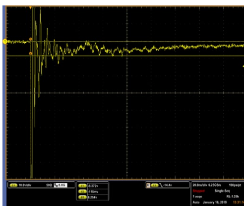
ISO10605 (C:330pF, R:330Ω) contact discharge plot at -8KV
