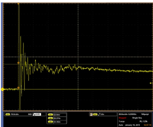
ISO10605 (C:330pF, R:330Ω) contact discharge plot at +8KV
