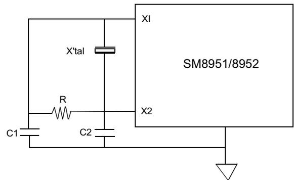
NOTE: Oscillation circuit may differs with different crystal or ceramic resonator in higher oscillation frequency which was due to each crystal or ceramic resonator has its own characteristics. User should check with the crystal or ceramic resonator manufacturer for appropriate value of external components.
