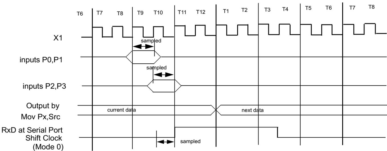
Timing Critical, Requirement of External Clock ( $V_{ss}=0.0V$  is assumed)
