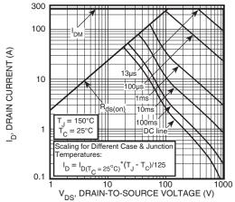
Figure 10, Maximum Forward Safe Operating Area
