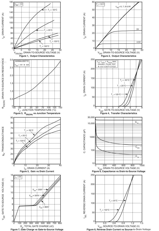
Figure 8, Reverse Drain Current vs Source-to-Drain Voltage
