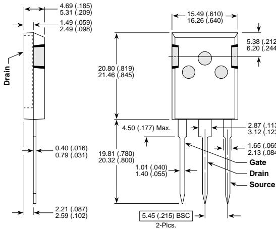
These dimensions are equal to the TO-247 without the mounting hole.
