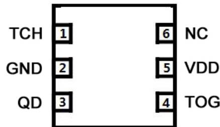
APS8233B, DFN6L (2\*2\*0.75mm), NMOS 开漏输出(QD), 16 秒
