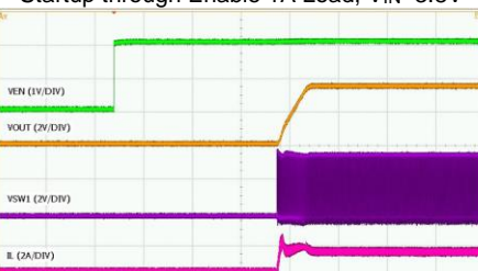
Startup through Enable 1A Load, V IN =3.8V
