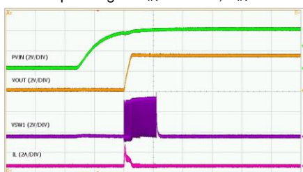
Startup through P VIN No Load, V IN =3.8V
