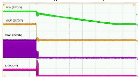
Shutdown through P VIN 1A Load, V IN =3V
