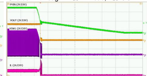
Shutdown through P VIN 1A Load, V IN =5.5V
