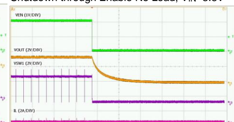
Shutdown through Enable No Load, V IN =3.8V
