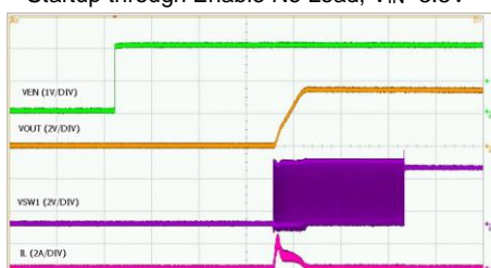
Startup through Enable No Load, V IN =3.8V
