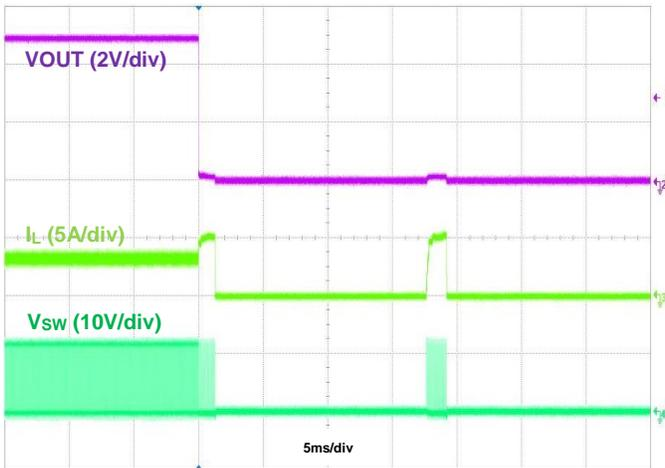
Figure 21. Output Short Protection, IOU = 3.5A
