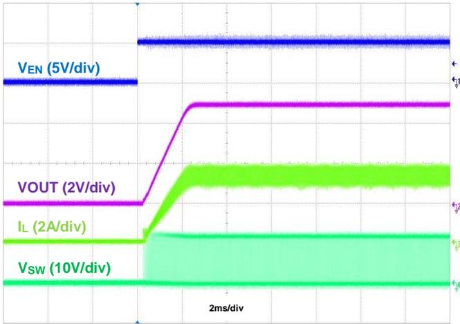
Figure 19. Startup Using EN, IOU = 3.5A
