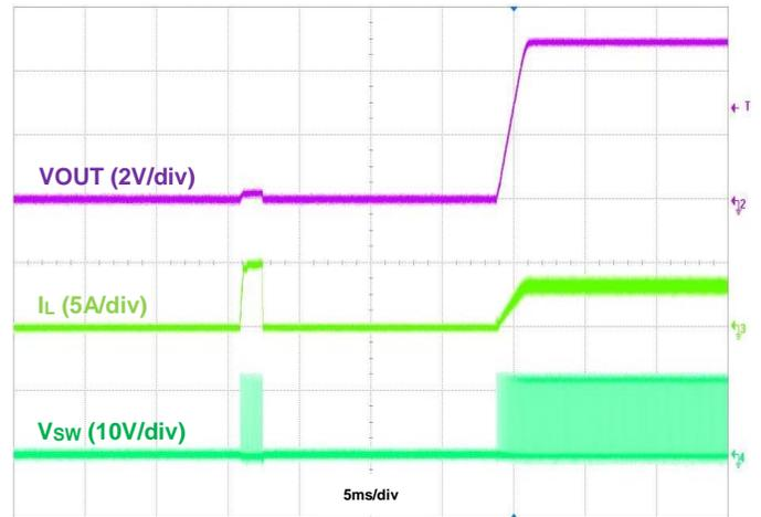
Figure 22. Output Short Recovery, IOU = 3.5A
