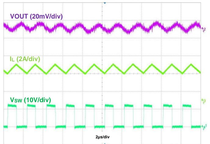
Figure 15. Output Voltage Ripple, IOU = 3.5A
