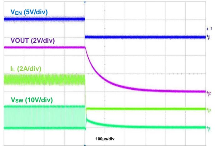
Figure 20. Shutdown Using EN, IOU = 3.5A
