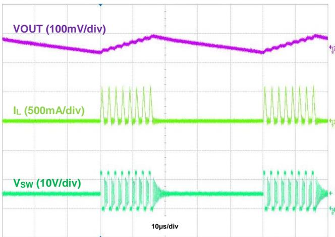
Figure 14. Output Voltage Ripple, IOU = 50mA
