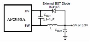
Figure 4 Add Optional External Bootstrap Diode to **Enhance Efficiency**
