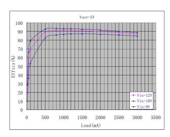
Figure 2. Typical Efficiency Curve
