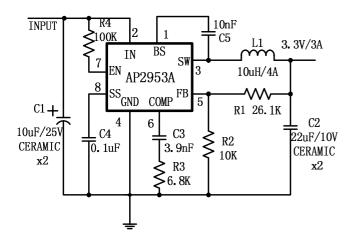
Figure 1. Typical Application Circuit
