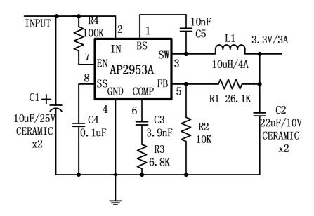
Figure 3—AP2953A with 3.3V output, 2X22uF Ceramic Output Capacitor
