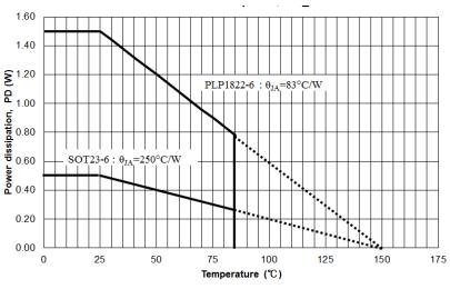
Figure 2. Maximum Power Dissipation
