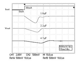
■  $C_L$ =1.0 $\mu$ F, 2.2 $\mu$ F, 4.7 $\mu$ F:  $I_{OUT}$ =30 $\Rightarrow$ 0mA
