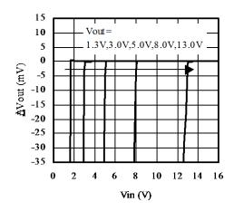
■ Regulation Point  $(2.1V \le V_{OUT(typ)})$
