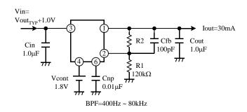
$V_{OUT(TYP)}$  =3.0V : R2=163.5k $\Omega$
