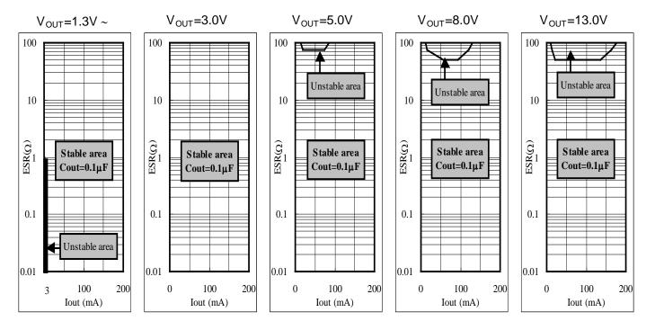
Figure 3. Stable operation area vs. voltage, current, and ESR
