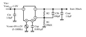
$V_{OUT(TYP)}$ =3.0V: R2=163.5 $k\Omega$
