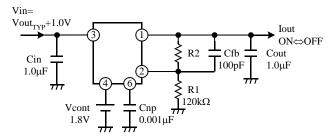
$V_{OUT(TYP)}$  =3.0V : R2=163.5k $\Omega$
