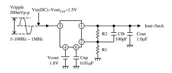
$$\begin{split} V_{\text{OUT(TYP)}} = & 1.3 \text{V: } \text{R1=120k}\Omega, \text{ R2=2.8k}\Omega \\ & 3.0 \text{V: } \text{R1=120k}\Omega, \text{ R2=163.5k}\Omega \\ & 5.0 \text{V: } \text{R1=120k}\Omega, \text{ R2=352k}\Omega \\ & 8.0 \text{V: } \text{R1=75k}\Omega, \text{ R2=397k}\Omega \\ & 13.0 \text{V: } \text{R1=51k}\Omega, \text{ R2=470k}\Omega \end{split}$$
