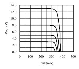
■ Load Regulation (V<sub>OUT(TYP)</sub> =3.0V)
