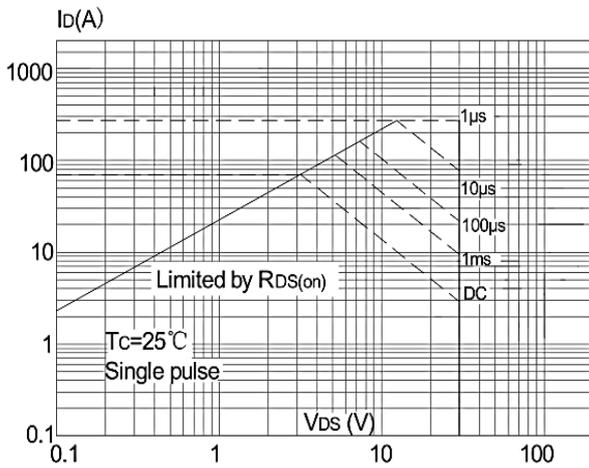
**Figure 9: Maximum Safe Operating Area vs. Case Temperature**
