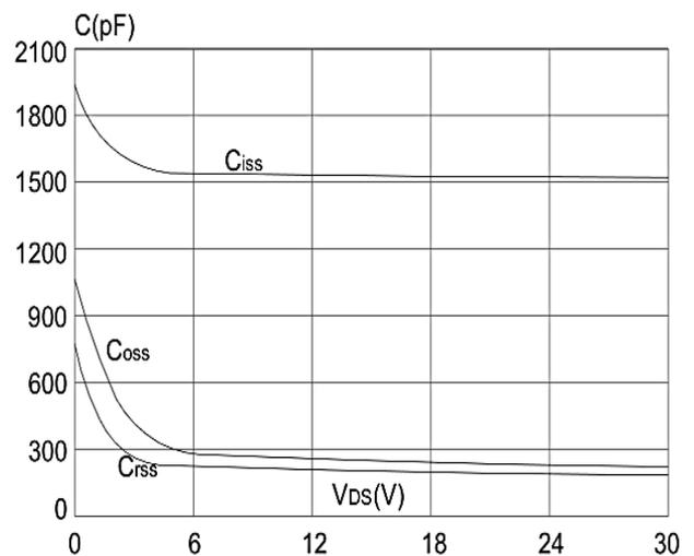
**Figure 6: Capacitance Characteristics**
