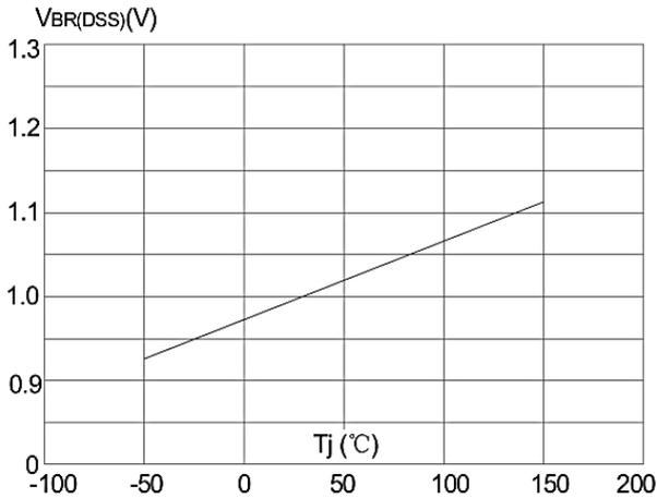
**Figure 7: Normalized Breakdown Voltage vs. Junction Temperature**
