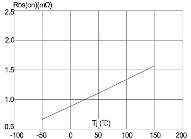
**Figure 8: Normalized on Resistance vs. Junction Temperature**
