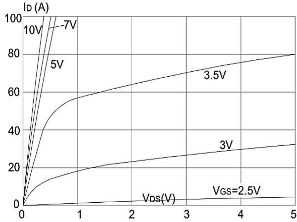
**Figure 1: Output Characteristics**
