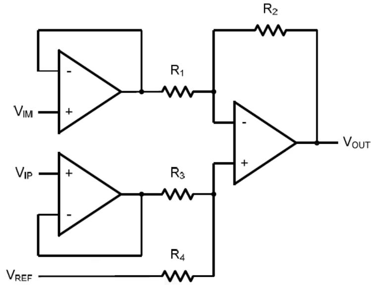
Figure 5. Instrument Amplifier
