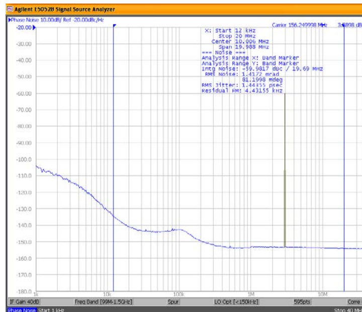
156.25MHz Input Clock with Bad Spur at 3MHz, Causing 1.4ps RMS Phase Jitter
