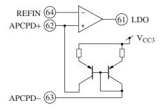
A current mirror circuit of which primary side is APCPD- is built-in. In case where output of secondary side is connected to APCPD+ and PD current for laser monitor is sunk to PD, the direction of current can be reversed by connecting the PD output to APCPD-.
