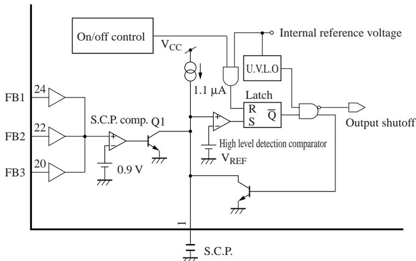
Figure 6. Short-circuit protection circuit
