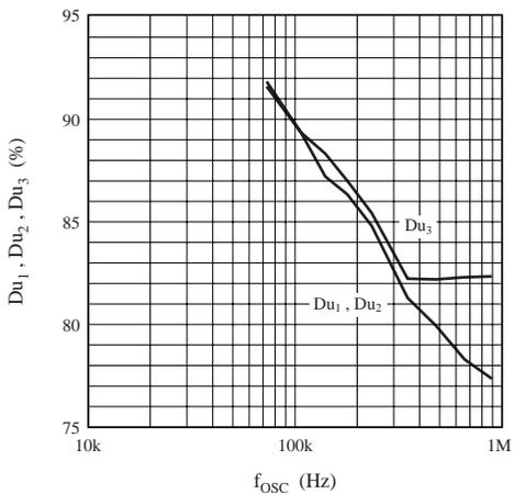
$f_{osc}$  — Maximum output duty ( $R_T = 33\text{ k}\Omega$ )
