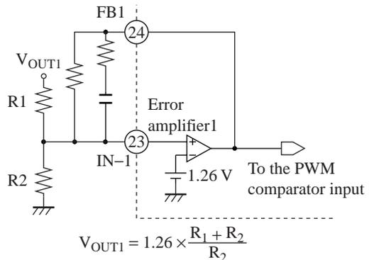
Figure 2. Connection method of error amplifier 1
