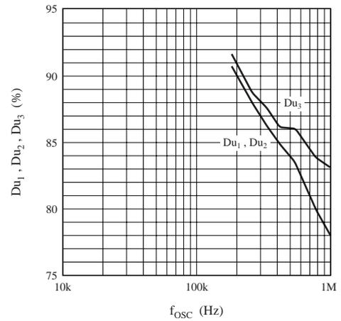
$f_{osc}$  — Maximum output duty ( $R_T = 7.5\text{ k}\Omega$ )
