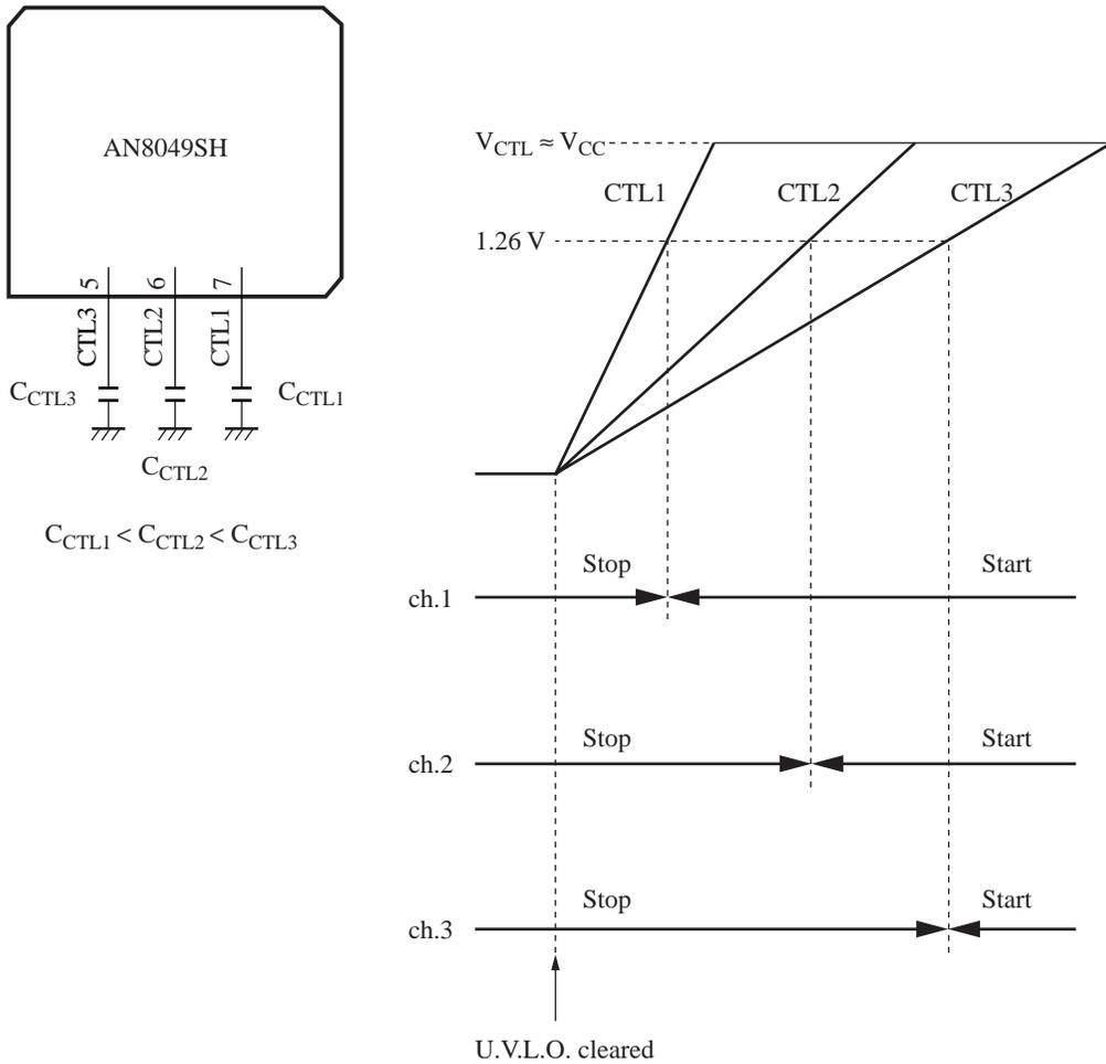
Figure 8. Sequential operation using external capacitors
