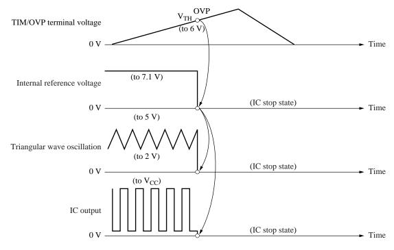
Figure 2. Explanation of OVP operation
