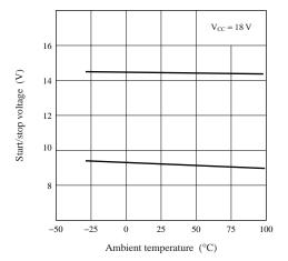
OVP operation threshold voltage characteristics
