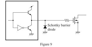
For the current capability, the peak current is major concern, and the particularly large current is not required normally: The power MOSFET which works as load on the output is capacitive load. Therefore, in order to drive it at high speed, the large peak current is required. However, after charge/discharge particularly large current is not required to keep that condition.
