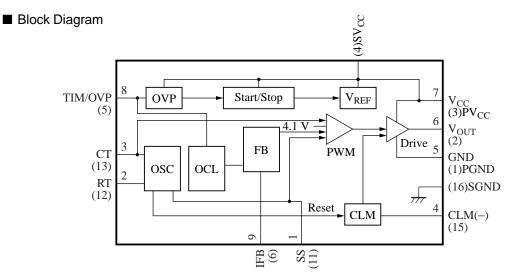
Note) The number in ( ) shows the pin number for the AN8022SB.
