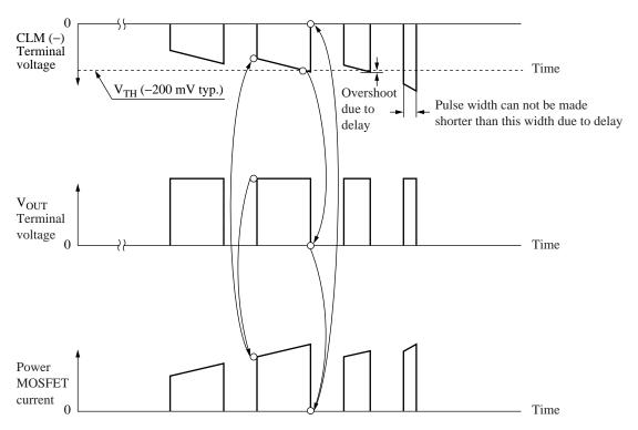
Figure 6. Pulse-by-pulse overcurrent detector operation waveform
