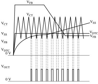
Figure 7. Soft start operation waveform
