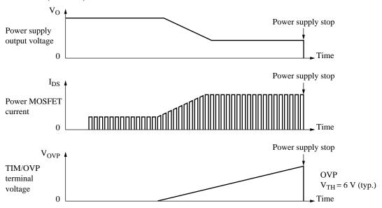
Figure 8. Timer latch basic operation
