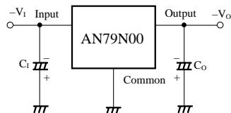
C<sub>i</sub> is connected when the input line is long. 2μF
